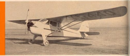
The Monocoupe 90-A, in production since 1927, was still being advertised in 1952, a record in longevity. The company had undergone reorganizations and name changes but the airplane was basically the same—its 65 h.p. increased to 145 h.p. and lines gradually refined. In 1941, the radial engine was replaced by a Franklin flat-four. Postwar models used Lycomings.
