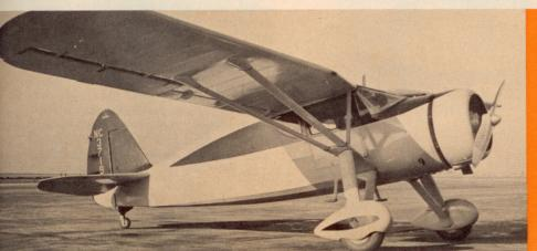
The Fairchild 24J of 1938 was a considerably refined version of the original "24" of 1933, a two-seater powered with either the 95 h.p. Cirrus or 125 h.p. Warner engine. The "24" developed through a three-place model to a four-place and standardized on two engines, the Warner radial and the inverted in-line Ranger. Both versions were in production for the Army through World War II and for the civilian market for a short time afterward. Many are still in use today as private-owner types.
